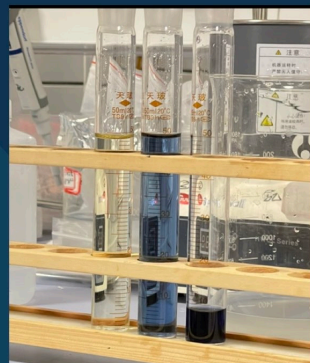
Fig. 6. Color change after adding the reagents, from left to right: after filtration, before filtration
